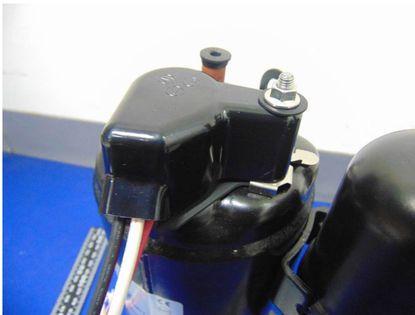
Picture No.4: Cover compressor
